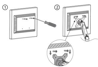
Recessed surface installation:Put spacers between headplate and monitor. Install the lower two screws and fasten the upper two screws.
